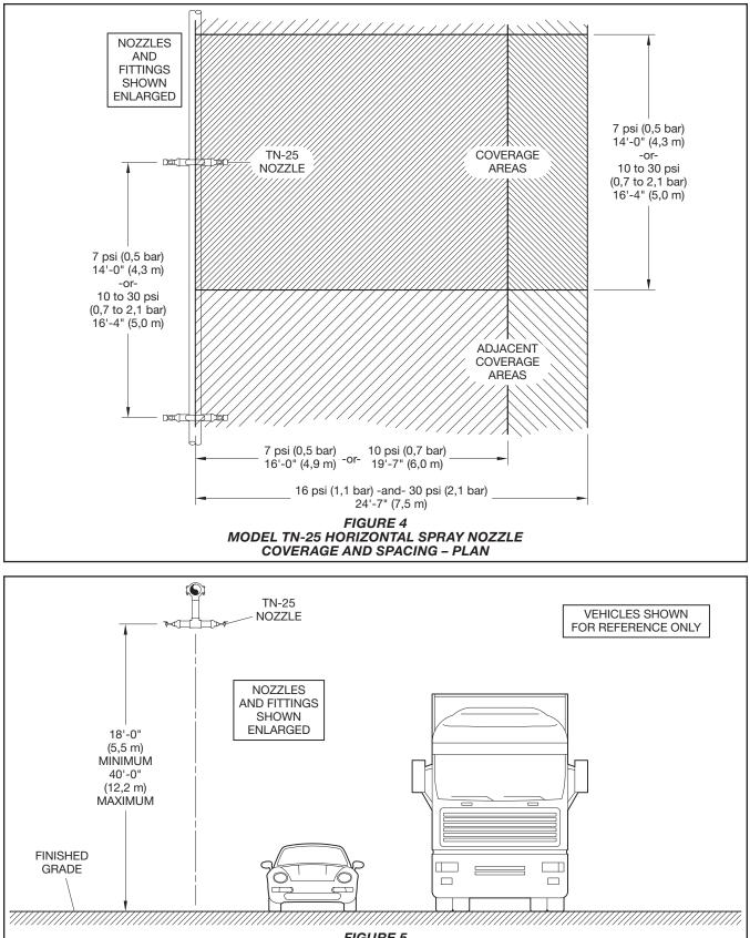
FIGURE 5 MODEL TN-25 HORIZONTAL SPRAY NOZZLE COVERAGE AND SPACING – ELEVATION
