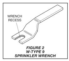
After installation, the sprinkler wrench flats and frame arms must be inspected and the wax coating retouched (repaired) whenever the coating has been damaged and bare metal is exposed. The wax coating on the wrench flats can be retouched by gently applying a heated 1/8 in. diameter steel rod to the areas of wax that have been damaged, to smooth it back over areas where bare metal is exposed.
